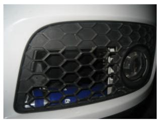
Carefully refit the front bumper cover but do not force this on. Note if any areas around the fog light fixings are contacting with the new twintercooler piping. If they are then mark the area and then remove the front bumper and trim these areas with a sharp knife, you may have to cut as per the pictures below however some cars may require no trimming at all in this area.
