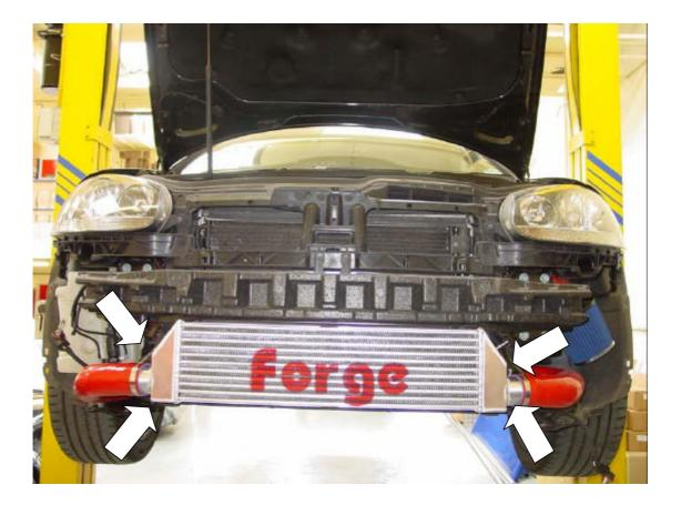
6/ Now fit the new 3 way hoses to each side of the intercooler and the new twintercooler using the hose clips supplied. Routing should be as pictured below. Tighten all hose clips securely once the hoses are fully positioned.
