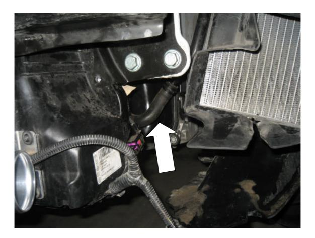
When installing the twintercooler silicon hose, you need to push the radiator pipe upward and let it lay over the silicon hose. Weave the pipe around to find the best layout
