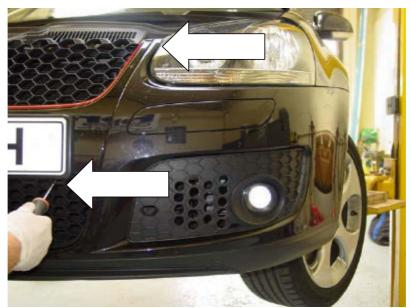
Now remove the 2x T30 screws that have been uncovered on the top edge of the bumper cover. Remove the 5x T20 Screws down each front wheel arch liner leading edge. Remove the 8x T20 screws from the lower edge of the front bumper.
