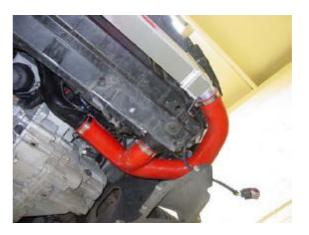
If you car equipped with DSG you might want to shorten the stock intercooler outlet silicon hose by 1-2 inches, to allow space from the black DSG metal pan.
