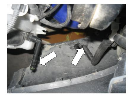
Disconnect both front fog light connections. The complete bumper cover is now ready to be removed by sliding the upper side fixings forward, remove the full bumper cover from the vehicle.
